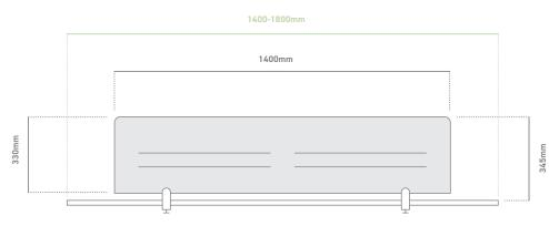
Black screen clamp brackets – no screen drilling required. Suits 15-25mm worktops.
