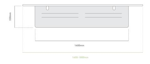
Black mounting brackets screw fix to the underside of the worktop.
