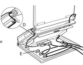
6. Loop a security lock (not included) around the laptop support (H) to secure L6 to a desk or laptop.
