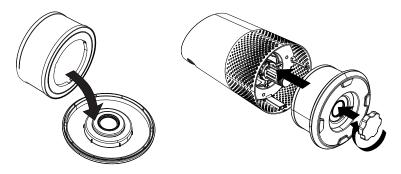
Secure filter on bottom cover and replace inside the purifier.
