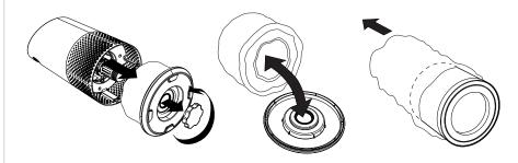
Unscrew bottom cover and remove plastic bag from filter.
